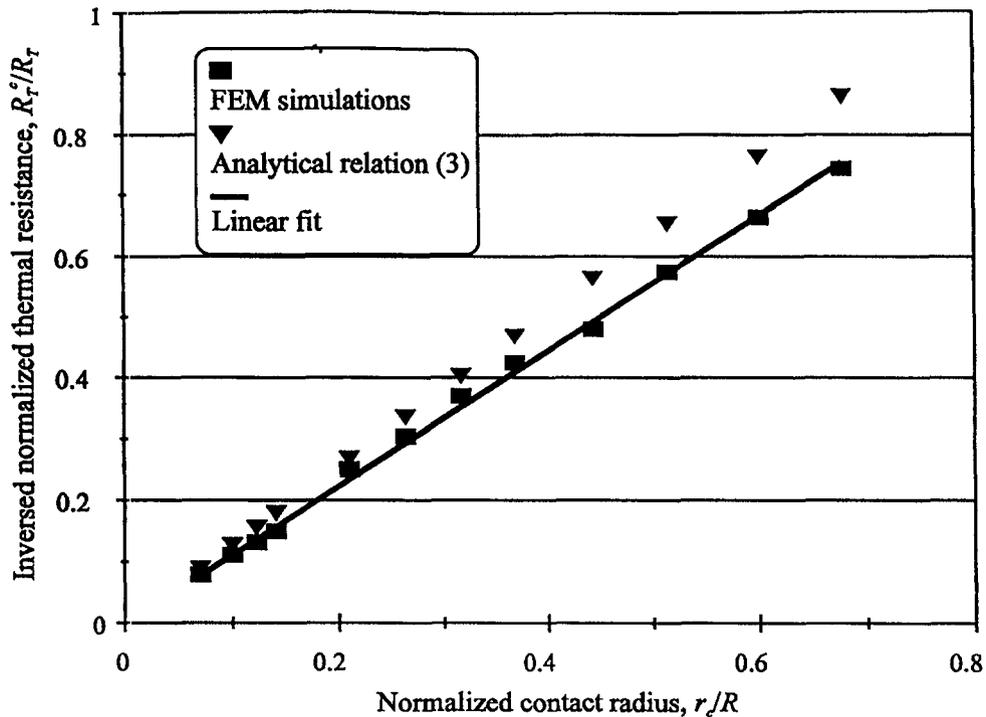
Fig. 2. Normalized thermal resistance as a function of normalized contact radius.
