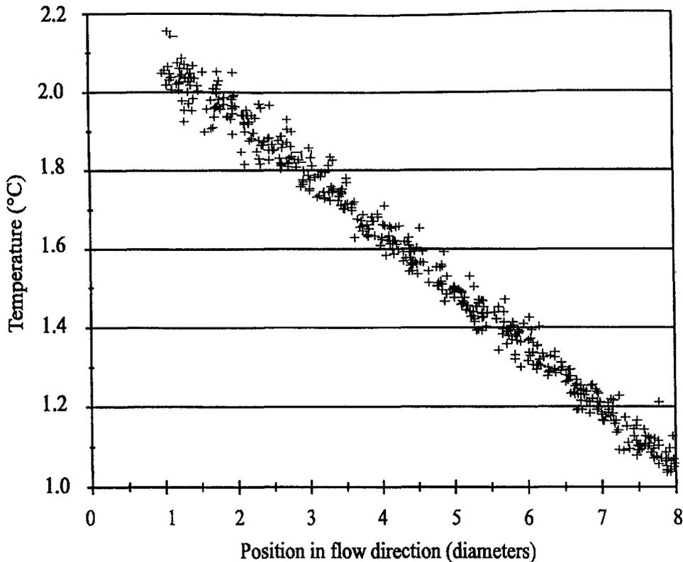
Fig. 5. Node (particle center) temperature distribution inside the packing as a function of position in the flow direction normalized with regard to particle diameter.
