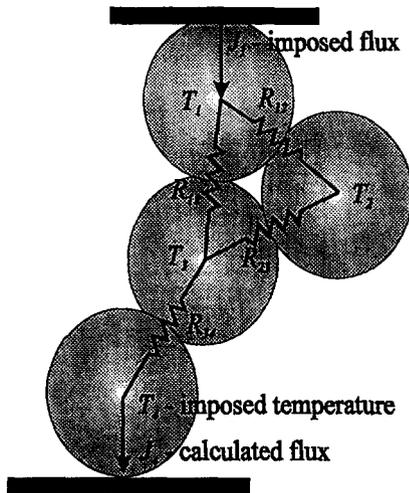
Fig. 3. Schematics of particle packing and equivalent thermal resistance network.
