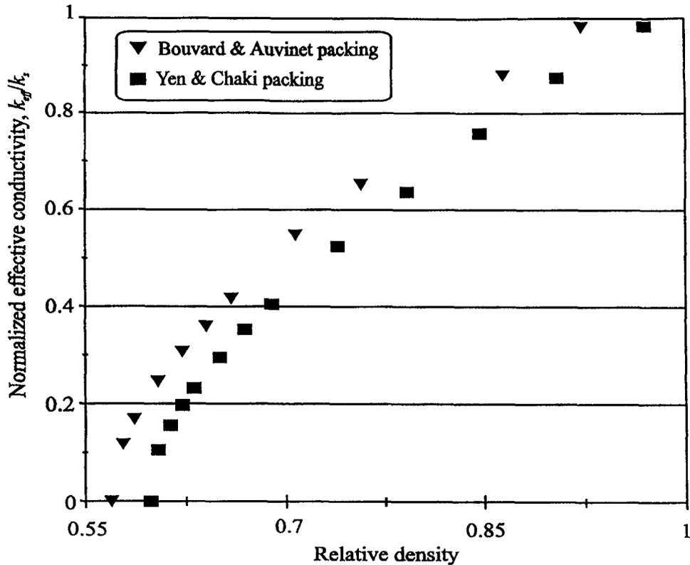
Fig. 6. Normalized effective conductivity for the two packings as a function of density.
