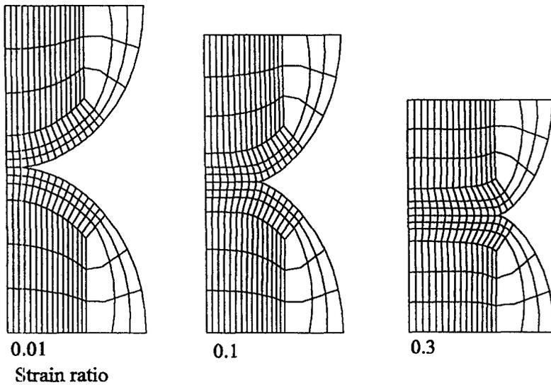
Fig. 1. Different meshes used for FEM calculations.
