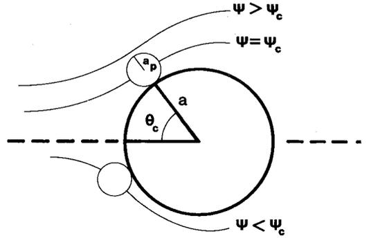
FIGURE 1. Deposition by interception. The angle of closest approach for a streamline in a boundary layer flow is  $\theta_c = 57.8^\circ$  for both cylinders and spheres.
