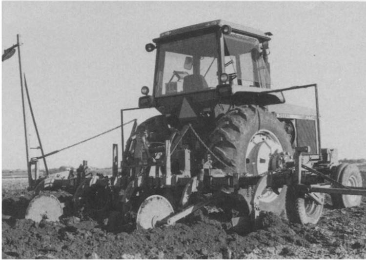
Fig. 1. Instrumented tractor with bedding implement. Axle strain gauge signals are transmitted by cables attached to arms on either side of rear axles. Note microcomputer to the left of operator seat. Terminal (above computer) is used by research personnel to communicate with the computer
