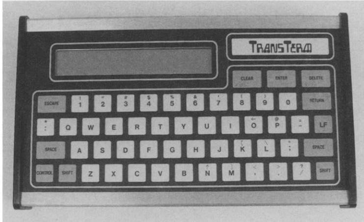
Fig. 5. Portable terminal used to communicate with the microcomputer
