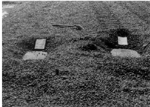
Figure 5. Exhumed GCL-2 specimens under the bulldozer track and 1.5 m away from the bulldozer track for test plot G-M ( H = 152 mm).
