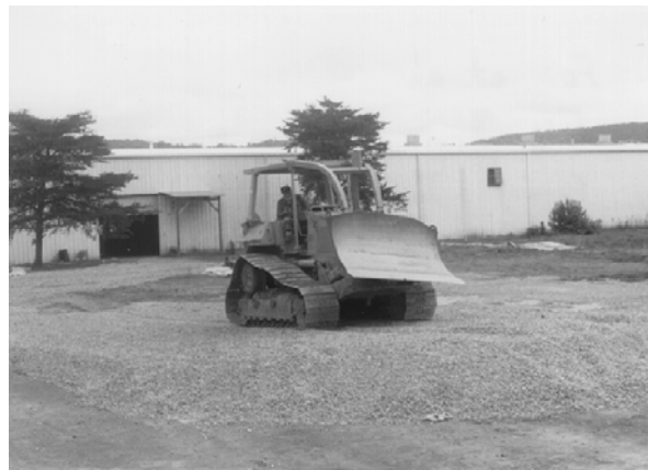
Figure 3. GCL trafficking for test plot G-M.
