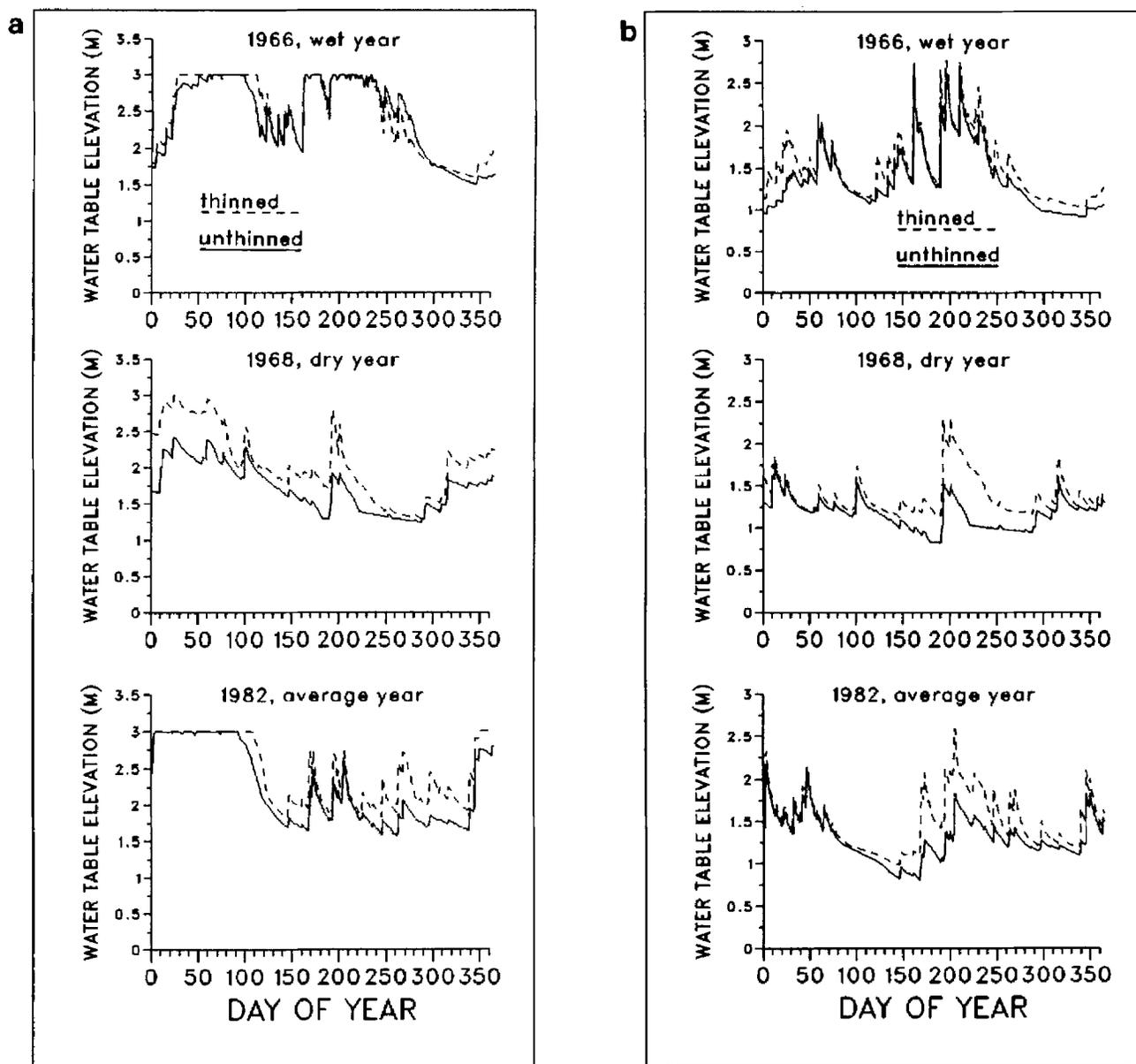
Figure 12. Effects of water management on water-table levels. a) No drainage. b) Controlled drainage. Controlled drainage allows for greater regulation over water-table levels, improving soil moisture conditions for tree growth and forest operations. Soil surface is at 3.0 m. Commercial thinning generally results in higher water tables with no drainage or controlled drainage. Data presented are DRAINMOD computer simulations (McCarthy 1990).
