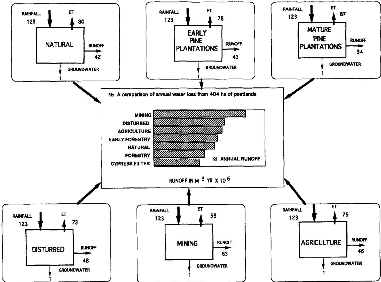
Figure 5. a) Hydrologic inputs and outputs by land-use type in cm/yr. Note: Output values were rounded to nearest whole number and may not exactly match inputs. b) Annual runoff ( $m^3 \times 10^6 \text{ yr}$ ) from a 404-ha block of peat-based wetlands under several land-use types as simulated for a 20-year period using the DRAINMOD model.
