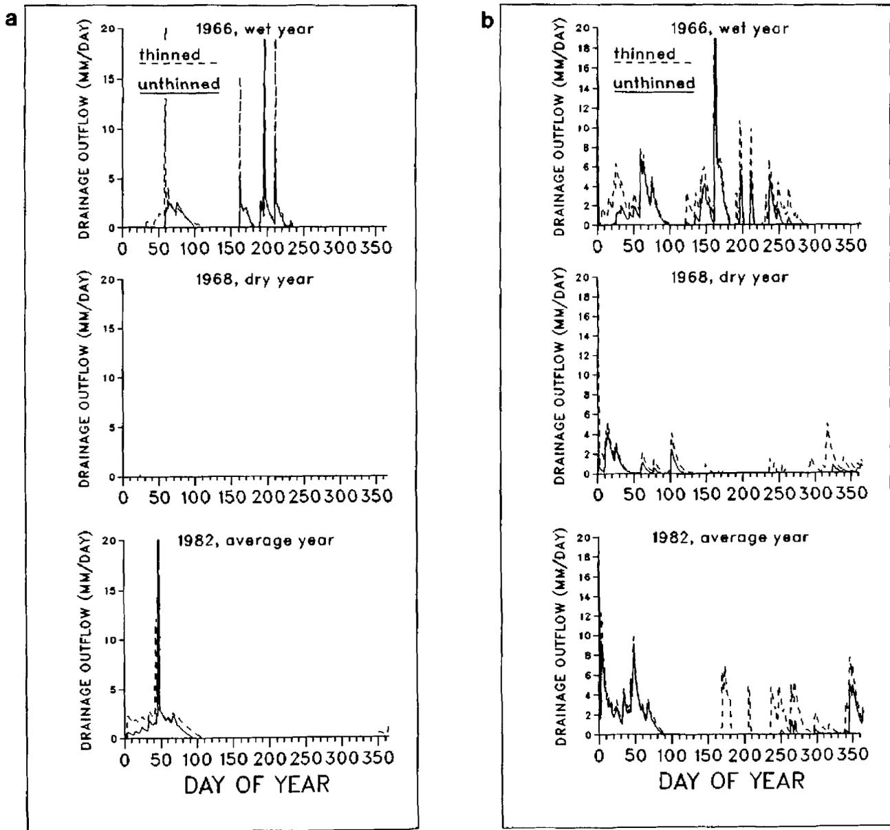
Figure 11. Effects of water management on drainage outflow from a forest watershed. a) No drainage. b) Controlled drainage. Controlled drainage systems can be designed to reduce the frequency of large peak flow rates (for this example, peak flow rates > 10 mm/day). Data presented are DRAINMOD computer simulations. Commercial thinning generally results in higher drainage outflows (McCarthy 1990).
