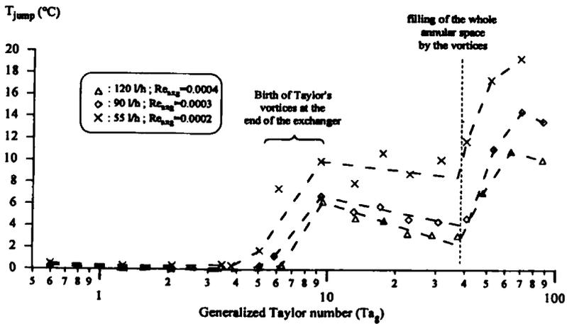
FIG. 4. EVOLUTION OF THE TEMPERATURE JUMP INSIDE THE INLET BOWL WITH RESPECT TO GENERALIZED TAYLOR NUMBER IN THE CASE OF COOLING OF THREE FLOWRATES OF GUAR GUM
