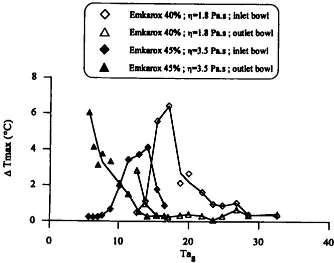
FIG. 3. THERMAL BEHAVIOR OF THE SSHE WITH RESPECT TO GENERALIZED TAYLOR NUMBER IN THE CASE OF HEATING OF EMKAROX SOLUTIONS; FLOWRATE: 160 l.h<sup>-1</sup> (EMKAROX 40%:  $Re_{sig}=0.159$ ; EMKAROX 45%:  $Re_{sig}=0.082$ )
