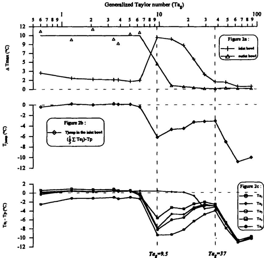
FIG. 2. EVOLUTION OF THE THERMAL BEHAVIOR OF THE SSHE WITH RESPECT TO GENERALIZED TAYLOR NUMBER IN THE CASE OF COOLING OF A GUAR GUM SOLUTION (2.3% WEIGHT); FLOWRATE: 120 l.h<sup>-1</sup> ( $Re_{axg} = 0.0004$ )
