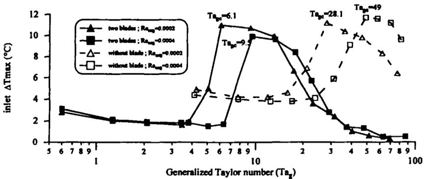
FIG. 6. EVOLUTION OF TEMPERATURE GRADIENT INSIDE THE INLET BOWL WITH RESPECT TO  $Ta_g$  AND NUMBER OF BLADES
