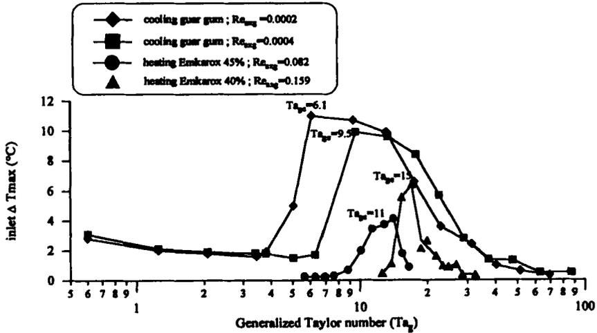
FIG. 5. EVOLUTION OF GENERALIZED TAYLOR NUMBER WITH RESPECT TO  $Re_{mg}$
