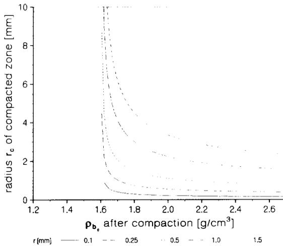
Fig. 3. Influence of body radius  $r$  on the affected radius  $r_c$  for an initial bulk density  $\rho_b = 1.6 \text{ g}/\text{cm}^3$ .
