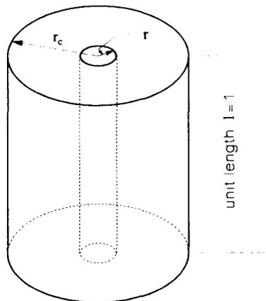
Fig. 1. Sketch of affected hollow cylinder ( $r$  = inner radius = outer radius of the affecting body,  $r_c$  = outer radius).
