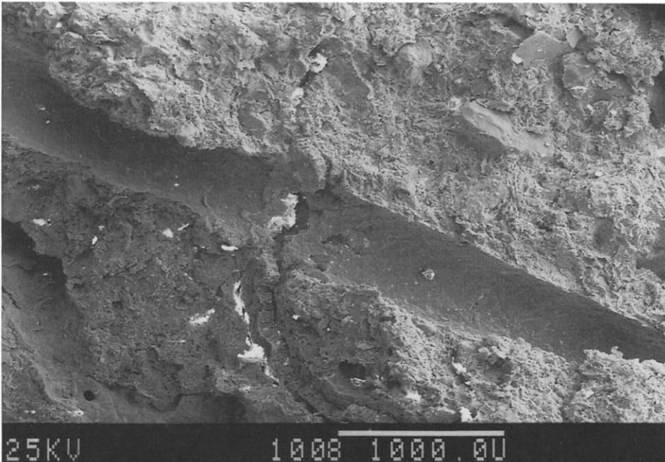
Fig. 2. SEM of the pathway of a 0.5 mm-probe showing the very thin layer compacted to minimum pore volume.
