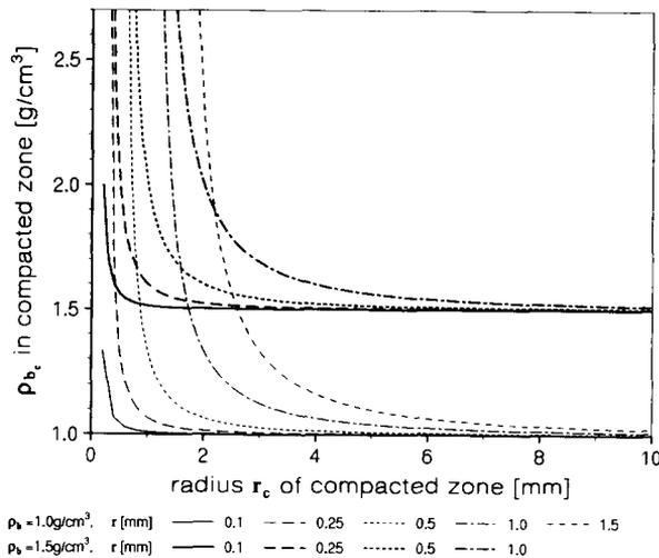
Fig. 5. Influence of affected radius  $r_c$  on  $\rho_{b_c}$  for different body radii  $r$  and  $\rho_b = 1.0$  and  $1.5 \text{ g/cm}^3$ .
