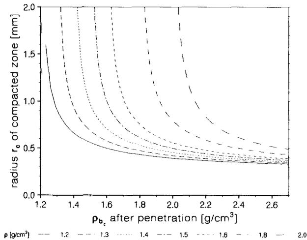
Fig. 4. Influence of initial bulk density  $\rho_b$  on the affected radius  $r_c$  for a body radius  $r=0.25$  mm.
