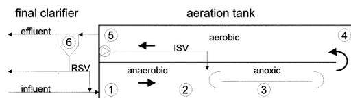
Fig. 1. Schematic process flux within the activated sludge tank and localization of the sampling sites. Abbreviations: ISV, internal sludge flow; RSV, return sludge flow; 1–5, sampling sites.
