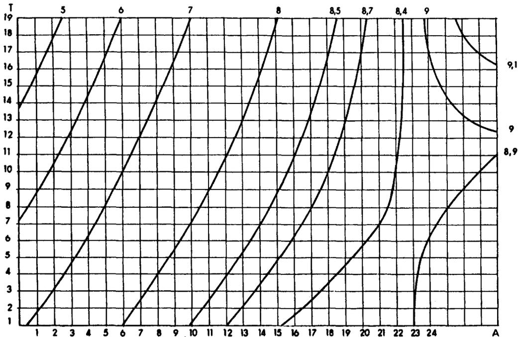
Fig. 5. Levels of methane produced with 2 cc of PVC and different concentrations of acetate (A) and sulphate (T).
