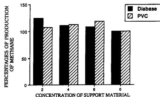
Fig. 1. Percentages of methane produced with different levels of diabase and PVC (concentrations are expressed as cc of support material/50 ml of sludge). The concentration 0 corresponds to the control conditions.
