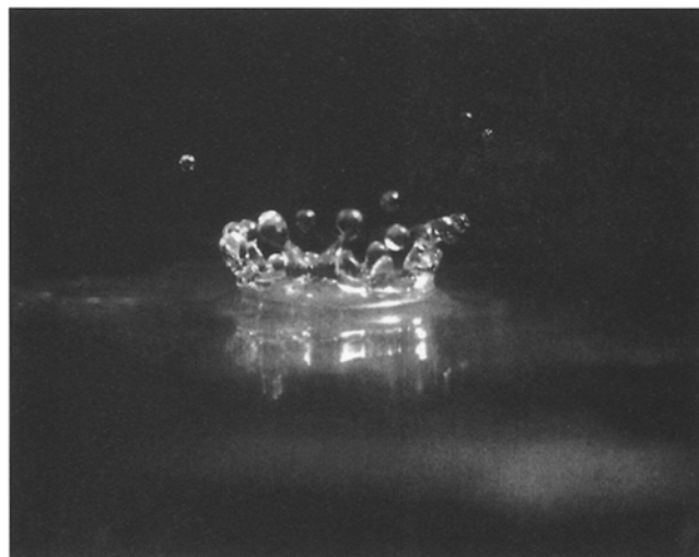
Fig. 7. Splash of a high viscosity drop (glycerine-water mixture 65%)
