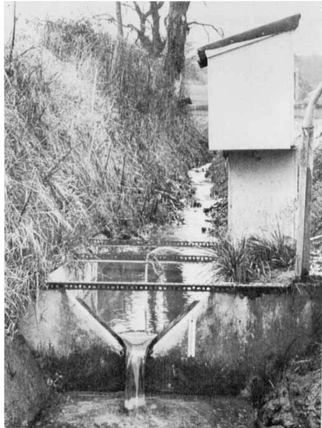
Figure 2. The 90° partially contracted V-notch weir and stage recorder housing
