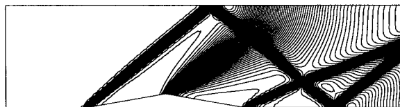
Figure 5. Density contours with \rho_{\min} = 0.6303 , \rho_{\max} = 2.0102 and an increment interval of 0.02.
