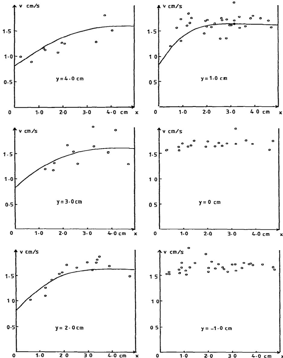
Fig. 9. Velocity profiles;  $\circ$  experimental values, — theoretical predictions.
