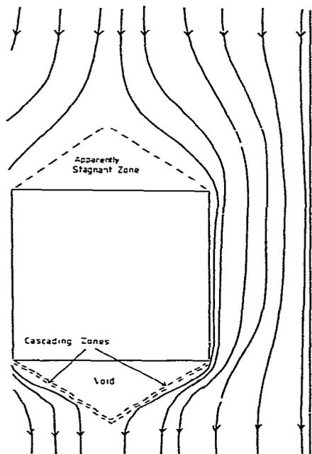
Fig. 4. Streamline pattern round square insert.
