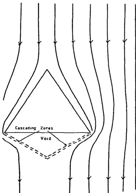
Fig. 6. Streamline pattern round triangular insert.
