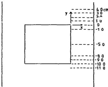
Fig. 8. Levels at which velocities were determined.
