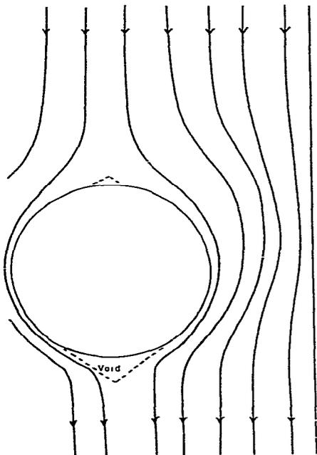
Fig. 5. Streamline pattern round circular insert.
