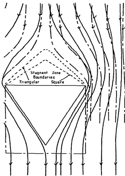
Fig. 7. Streamline patterns round square and triangular inserts; - - - square insert, — triangular insert.
