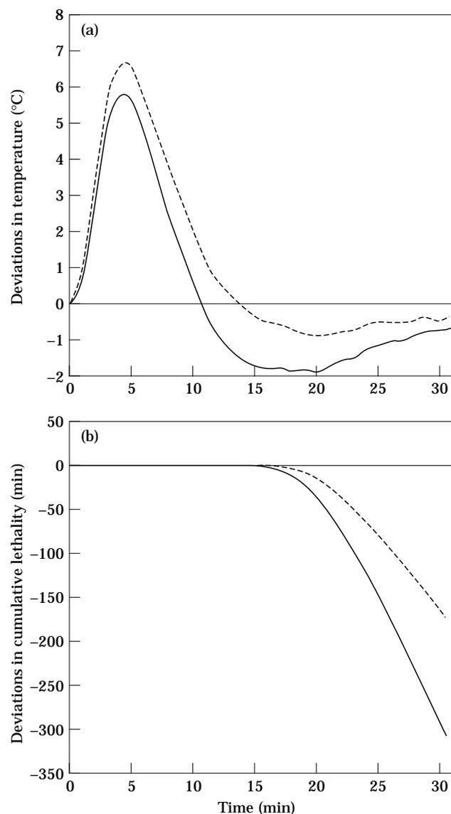
**Fig. 1** Comparisons of temperature histories and cumulative lethality between experiment and simulation: (a) the deviations of the simulated temperature history from the experimental one and (b) the deviations of the simulated cumulative lethality from the experimental one by using the least square method (—) and the optimization method (---) at one stage heating approximation
