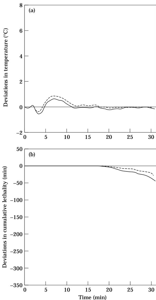
**Fig. 2** Comparisons of temperature histories and cumulative lethality between experiment and simulation: (a) the deviations of the simulated temperature histories to the experimental one and (b) the deviations of the simulated cumulative lethality to the experimental one by using the least square method (—) and the optimization method (---) at two stage heating
