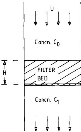
Fig. 1. Granular bed filter (schematic).
