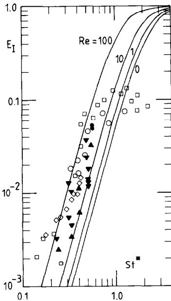
Fig. 5. Comparison of data for efficiency of inertial capture with correlation of D'Ottavio and Goren [28], evaluated for  $\epsilon = 0.38$  when  $Re_c = 0$ .
