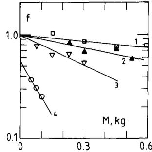
Fig. 3. Penetration  $f$  of di-ethyl hexyl sebacate aerosol through beds of closely sized glass beads as function of bed mass  $M$  in bed of diameter 7.62 cm. Data of Thambimuthu [23].
