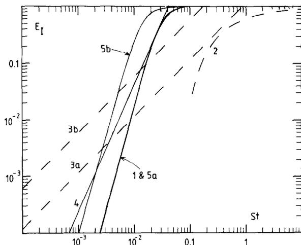
Fig. 7. Comparison of empirical and theoretical results for efficiency of inertial capture with  $\epsilon = 0.4$ . 1, Equation (17) (empirical); 2, Paretzky *et al.* [41] (cell model); 3, Pendse and Tien [20] (constricted tube model) (a)  $Re_c = 0$ ; (b)  $Re_c = 100$ ; 4, Goren [42] (empirical); 5, D'Ottavio and Goren [28] (empirical) (a)  $Re_c = 0$ ; (b)  $Re_c = 100$ .
