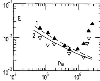
Fig. 4. Capture efficiency  $E$  for di-ethyl hexyl sebacate aerosol on glass beads as function of Peclet number  $Pe$ ; data of Thambimuthu [23] with  $D = 306 \mu\text{m}$ . 1, Downflow; 2, upflow; curves show total capture efficiency by diffusion, gravitational settling and direct interception, evaluated using expressions in the Table.
