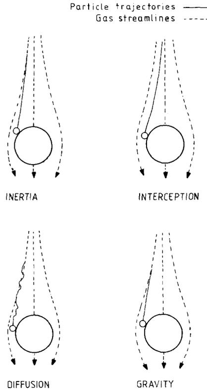
Fig. 2. Mechanical capture processes (schematic).
