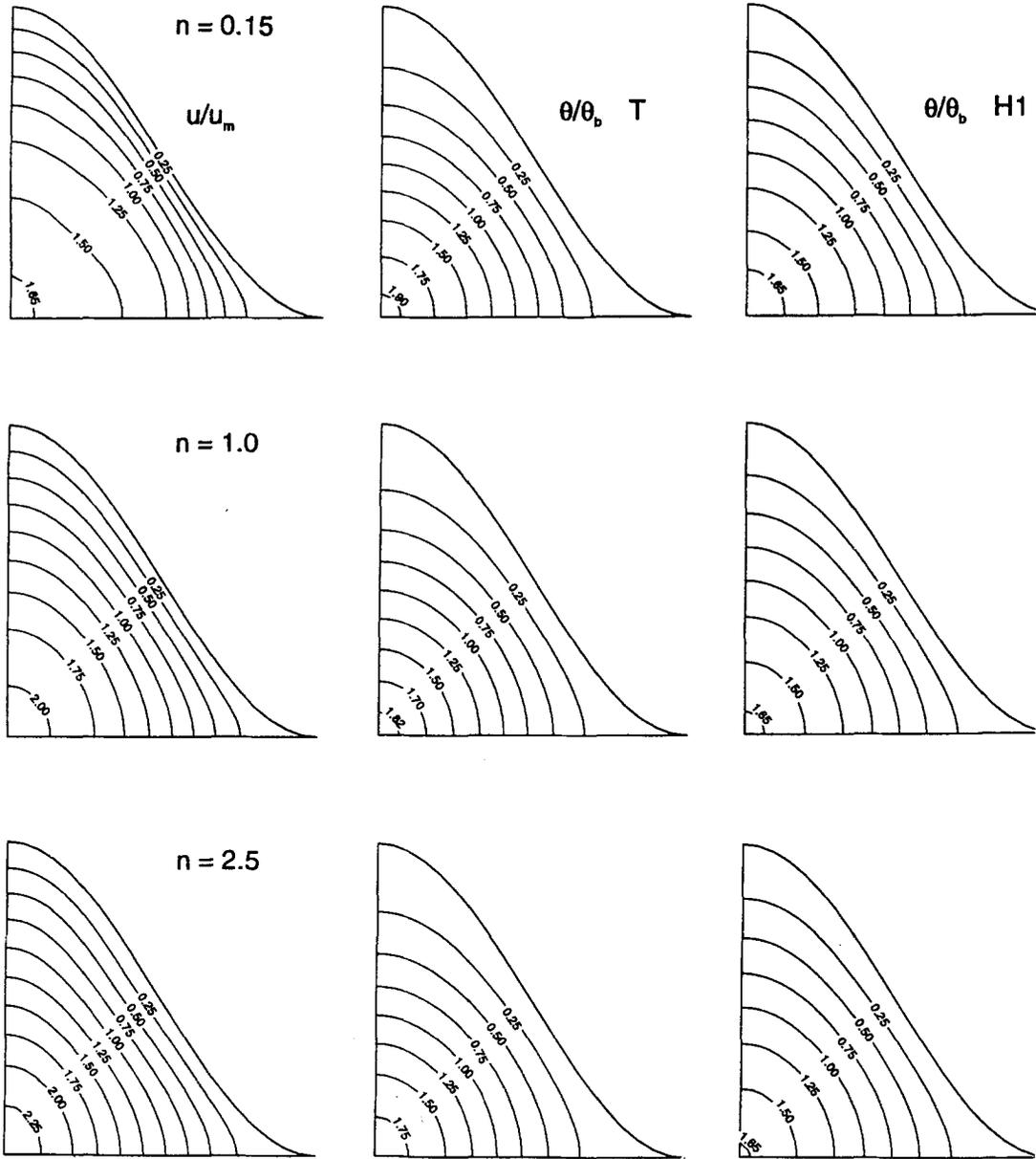
Fig. 2. Axial velocity ( $u/u_m$ ) contours and isotherm ( $\theta/\theta_b$ ) maps for  $n = 0.15, 1.0$  and  $2.5$  in a double-sine duct with  $\gamma = 1.0$ .
