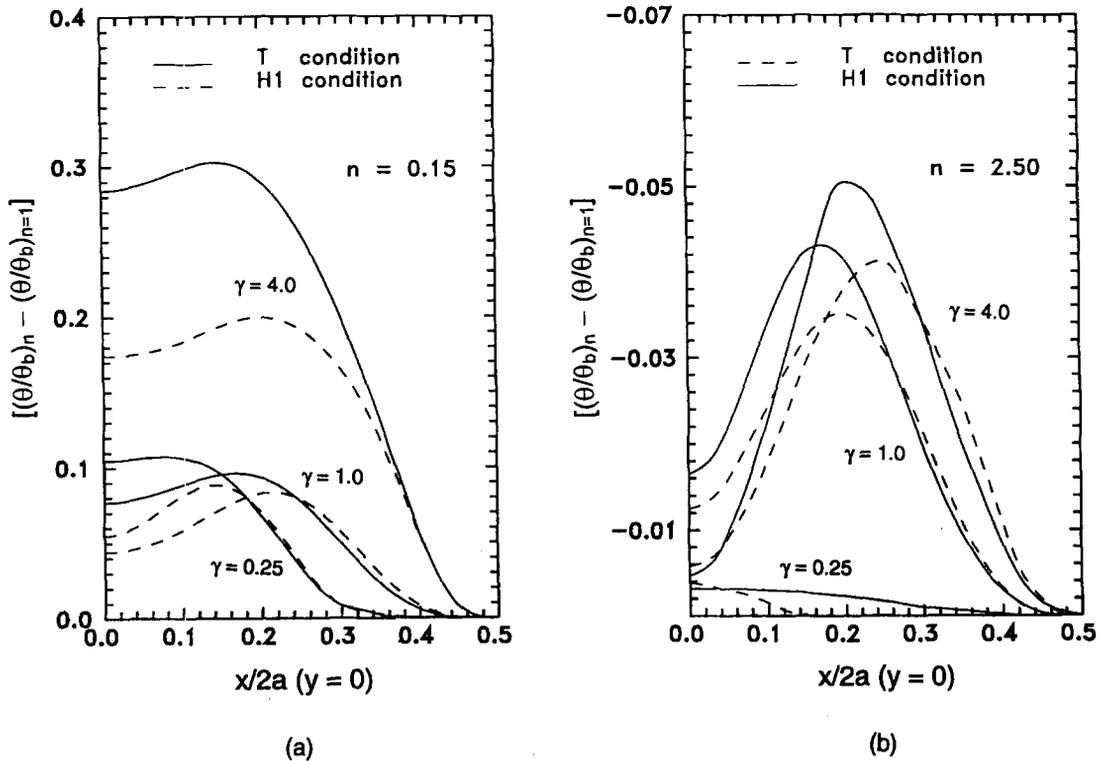
Fig. 4. Effect of flow behavior index on the mid-plane ( $y = 0$ ) temperature difference  $[(\theta/\theta_b)_n - (\theta/\theta_b)_{n=1}]$  distribution under T and H1 boundary conditions: (a) for  $n = 0.15$  and (b) for  $n = 2.5$ .
