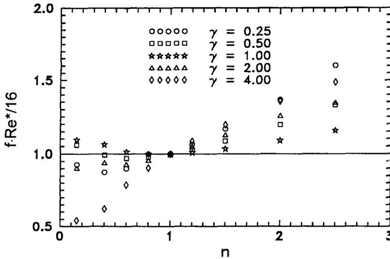
Fig. 6. Comparison of present results with  $fRe^*$  predictions of Kozicki *et al.* [22] for fully developed laminar flows with different flow behavior index  $n$  in double-sine ducts.
