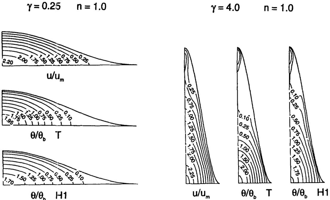
Fig. 3. Axial velocity ( $u/u_m$ ) contours and isotherm ( $\theta/\theta_b$ ) maps for  $n = 1.0$  in double-sine ducts with  $\gamma = 0.25$  and  $4.0$ .
