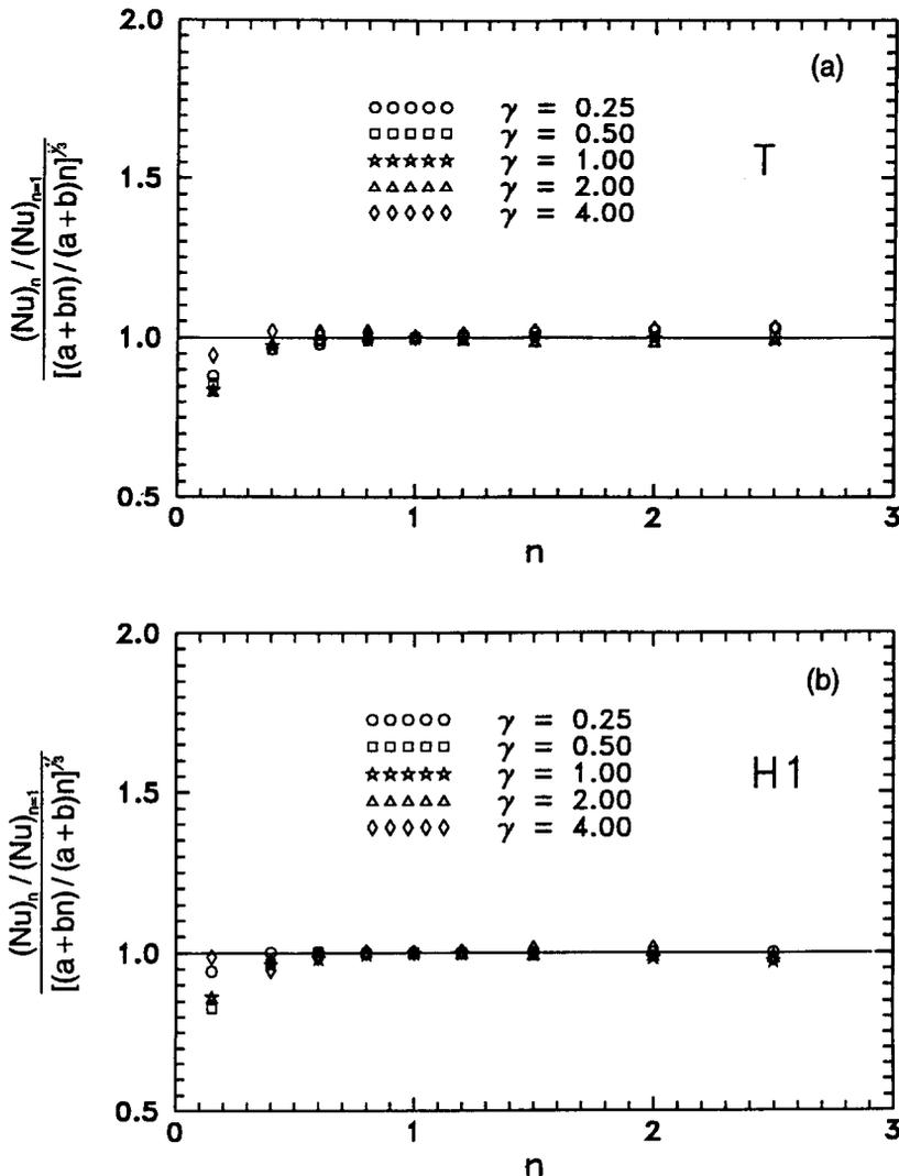
Fig. 7. Effectiveness of Cheng [13] parameter for correlating  $Nu$  in double-sine ducts: (a) for **T** and (b) for **H1** boundary conditions.
