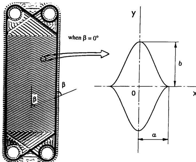
Fig. 1. Flow cross-section geometry and coordinate system for a double-sine shaped duct in typical chevron plate ( $\beta = 0^\circ$ ) passages.
