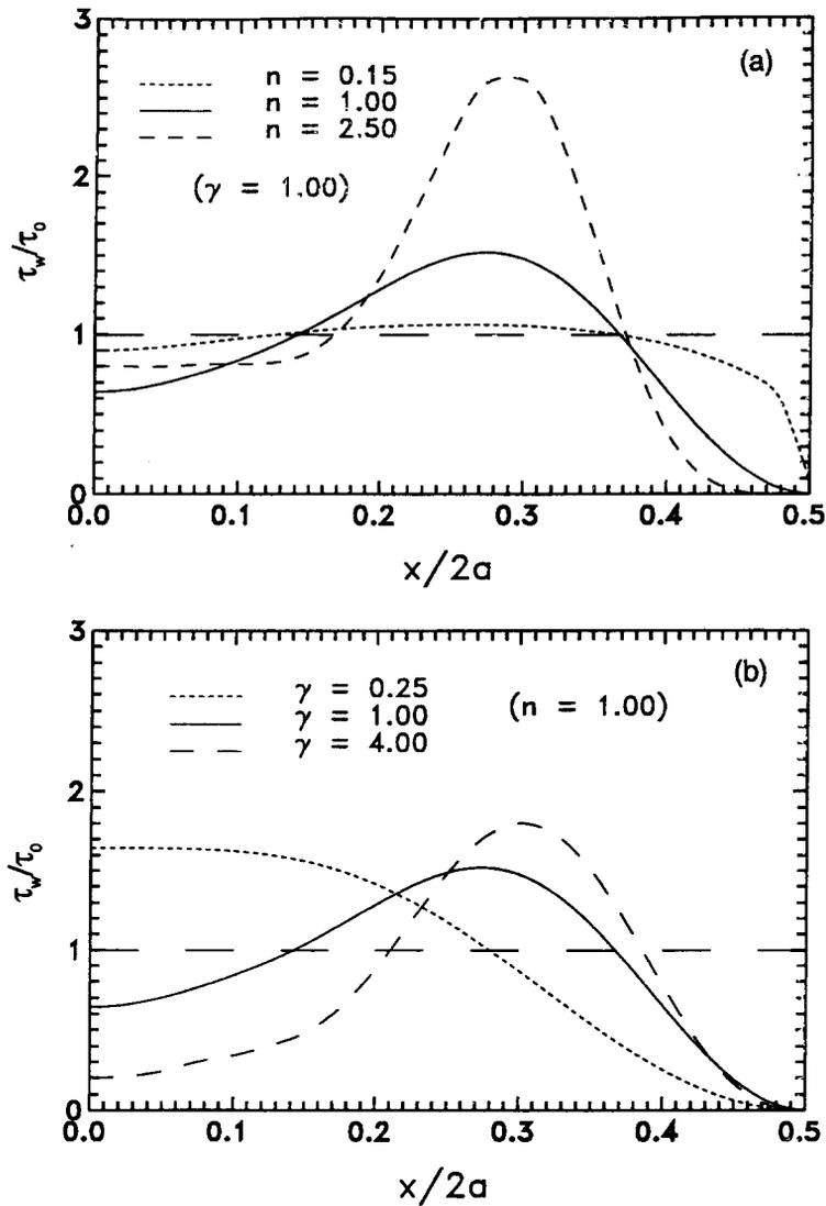
Fig. 5. Wall shear stress distribution ( $\tau_w/\tau_0$ ) in double-sine ducts: (a) variation with  $n$  and (b) variation with  $\gamma$ .
