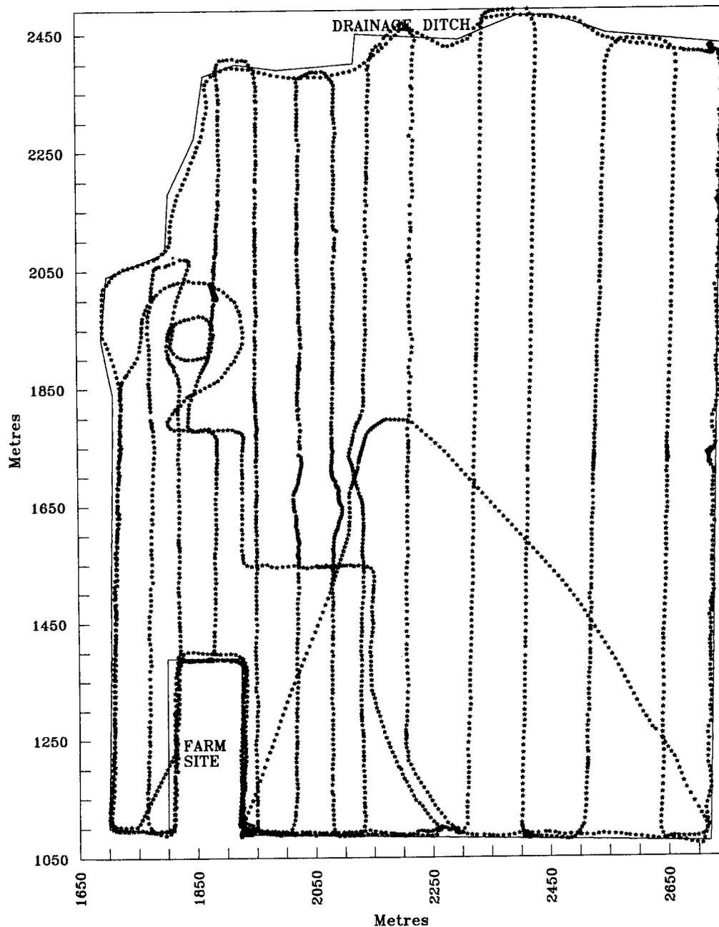
Fig. 2. EM-DGPS survey pattern, Stettler, 23 September 1992.
