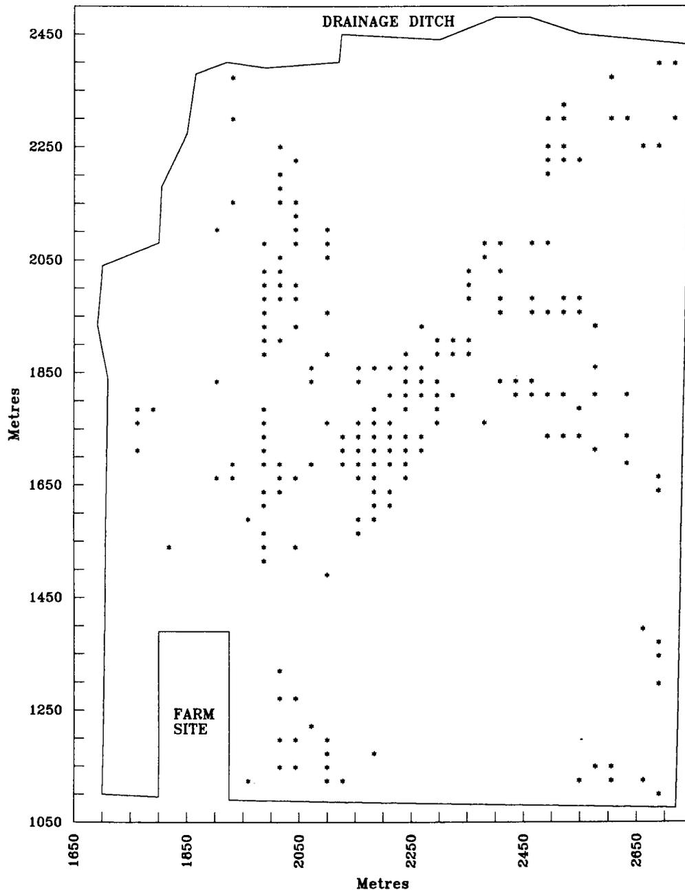
Fig. 8. Differences between EM surveys at 25 and 50 m line spacings. Points where the difference exceeds  $2 \text{ dS m}^{-1}$  are shown. Stettler survey, 23 and 24 September 1992.
