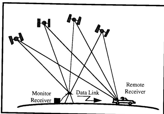
Fig. 1. GPS in the differential mode of operation. The data link is required when DGPS is used in real time.
