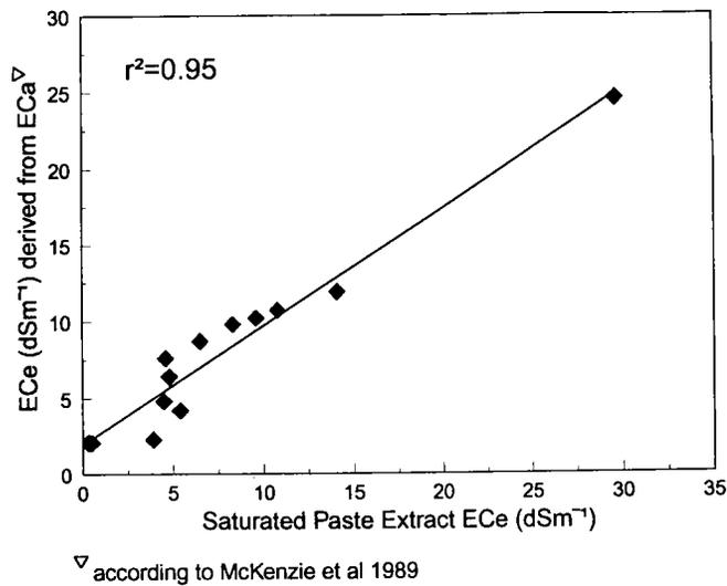
**Fig. 9.** Comparison of  $EC_e$  values from soil sample analysis and EM38 measurements, Stettler survey, September 1992.
