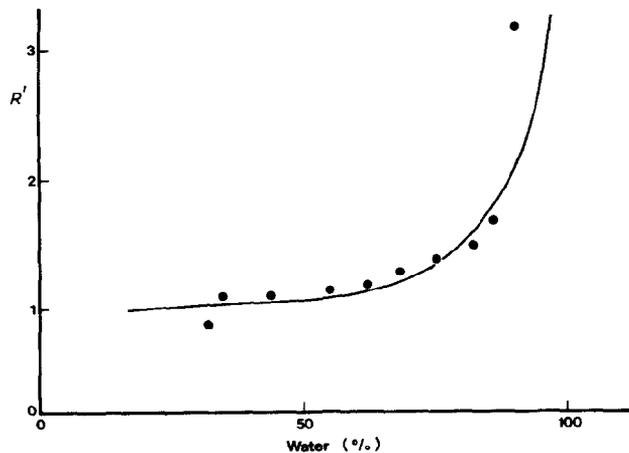
Fig. 3. Plot of F.t.-i.r. band ratio,  $R'$ , versus water content for drying wheat-starch gel. See text for the definition of  $R'$ .
