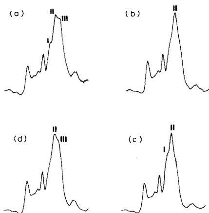
Fig. 1. I.r. spectra (1250–850 cm<sup>-1</sup>) of wheat starch (a) in cold water, (b) after gelatinisation at 90°, (c) gel stored at 1° in sealed cell for 21 days, (d) gel stored under drying conditions. Vertical axes in absorbance.
