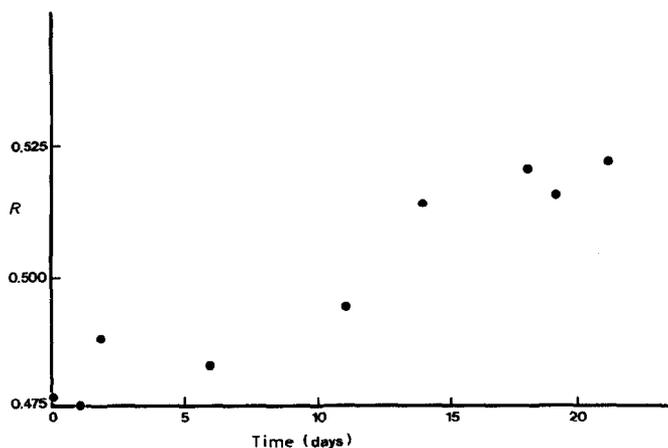
Fig. 2. Plot of F.t.-i.r. band ratio,  $R$ , versus time (days) for retrogradation of stored wheat-starch gel. See text for the definition of  $R$ .
