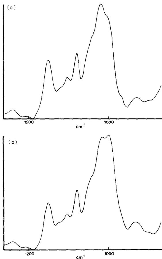
Fig. 4. I.r. (ATR) spectra of bread in the starch region ( $1250\text{--}850\text{ cm}^{-1}$ ): (a) fresh bread, (b) partially dried, stale bread. Vertical axes in absorbance.
