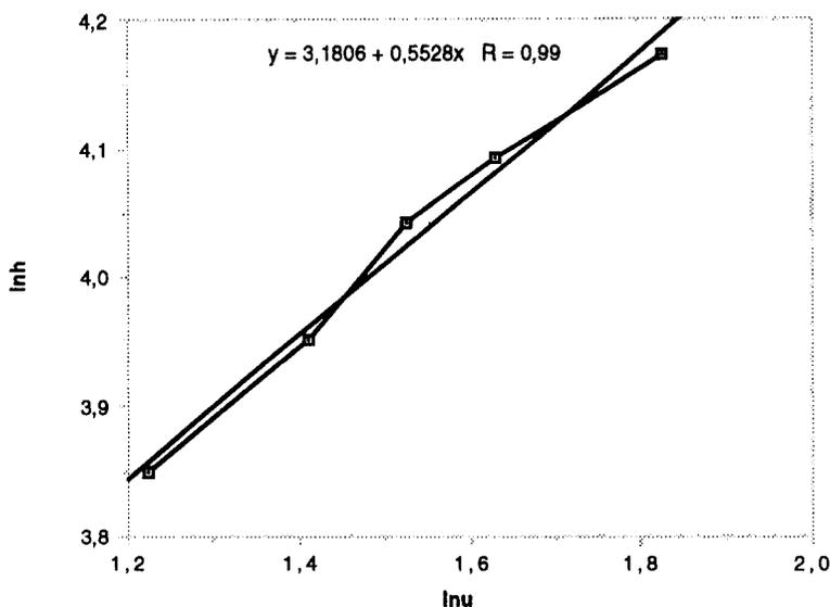
FIG. 3. REGRESSION ANALYSIS OF THE RELATIONSHIP HEAT TRANSFER COEFFICIENT ( $h$ ) - AIR FLOW RATE ( $u$ ), IN THE TURBULENT REGION ( $u$  is in m/s and  $h$  in W/m<sup>2</sup>K)
