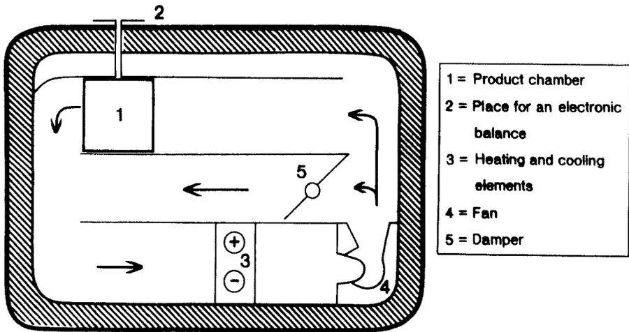
FIG. 1. A SCHEMATIC DIAGRAM OF THE THAWING TUNNEL
