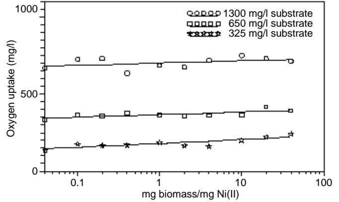
Fig. 4 Oxygen uptake versus biomass-to-metal ratio
