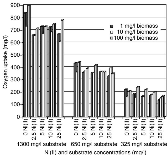
**Fig. 1** Oxygen uptake values at different substrate, Ni(II) and biomass concentrations
