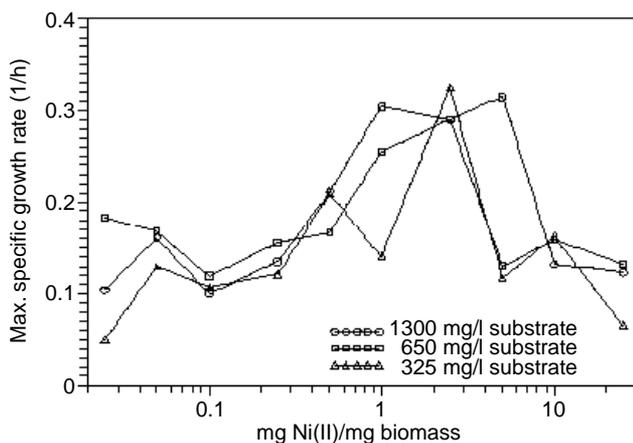
Fig. 5 Maximum specific growth rate versus Ni(II)/biomass ratio
