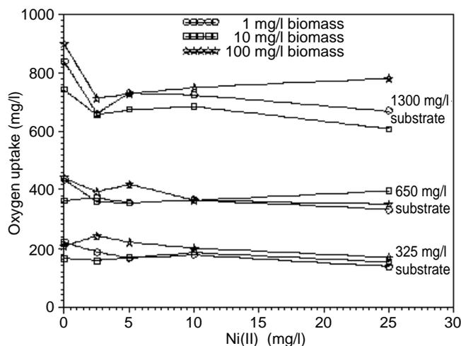
**Fig. 2** Oxygen uptake versus Ni(II) graph at different biomass and substrate concentrations
