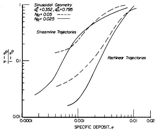
FIG. 6. Effect of particle size on simulation.
