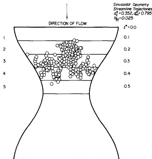
FIG. 11. Typical deposit pattern for streamline trajectories, elevation.
