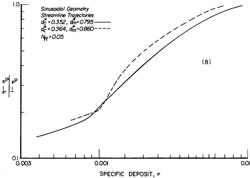
FIG. 5. Effect of unit cell dimensions on simulation.
