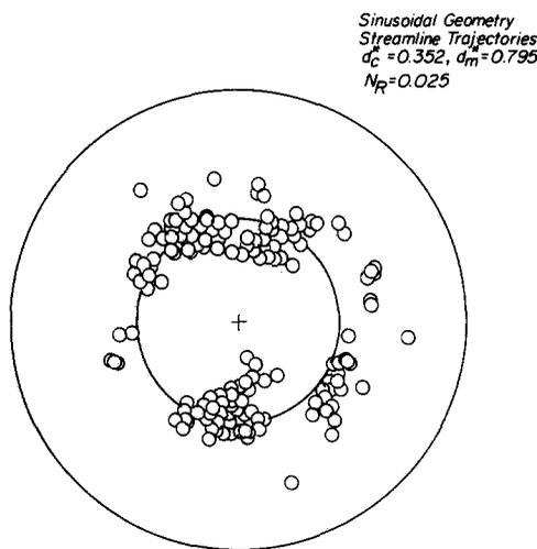
FIG. 10. Typical deposit pattern for streamline trajectories, plan.
