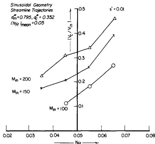
FIG. 9. Collection efficiency of various size fractions of polydisperse suspension.
