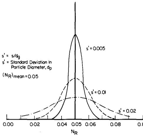
FIG. 7. Normal probability distribution function for particle size distribution.
