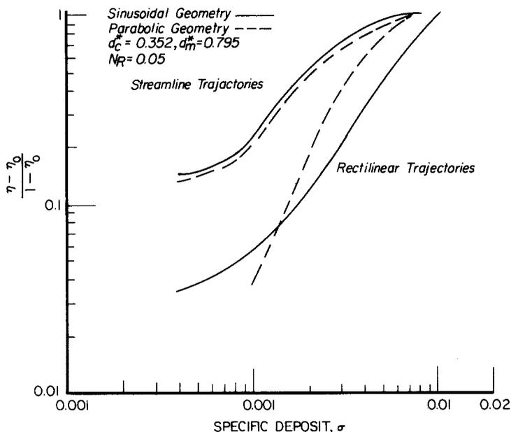
FIG. 4. Effect of tube geometry on simulation results.
