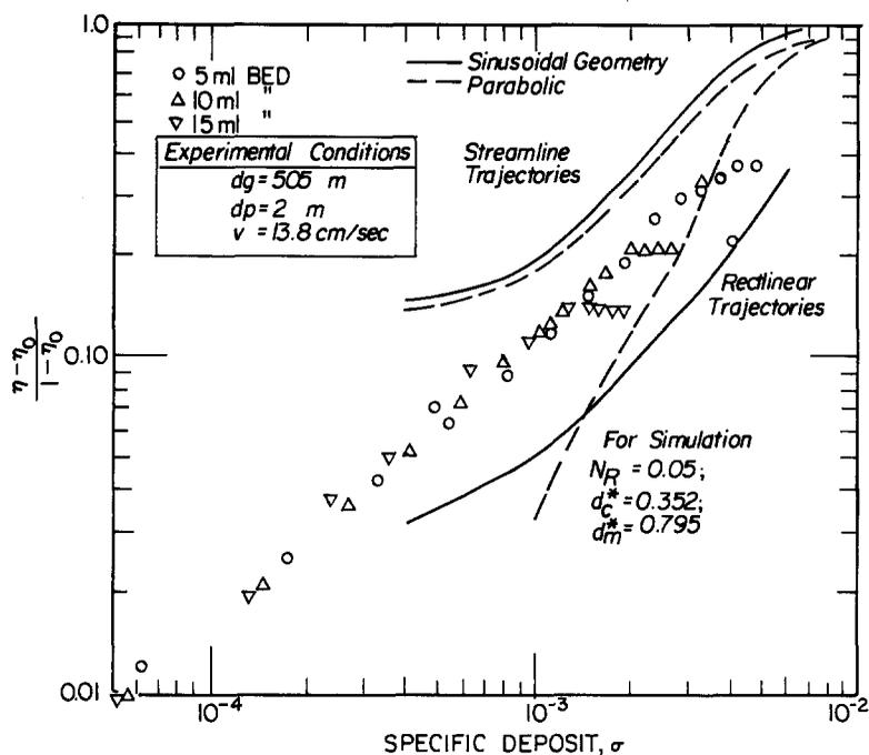
FIG. 13. Comparison between simulation model (Pendse, 1979) with experiments (Pannu, 1980).
