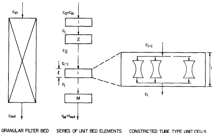
FIG. 1. Schematic representation of a granular filter bed.
