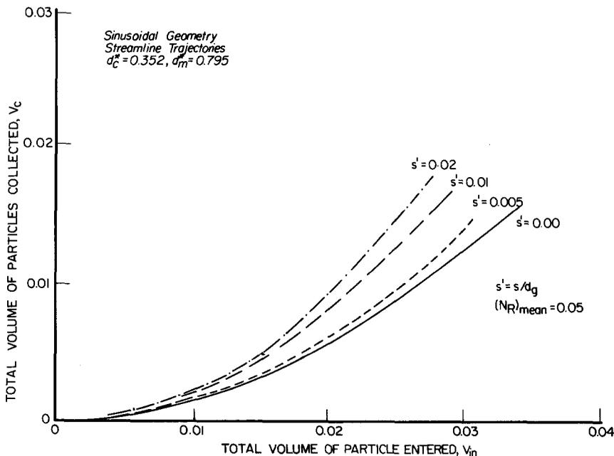
FIG. 8. Effect of particle size distribution on deposition.
