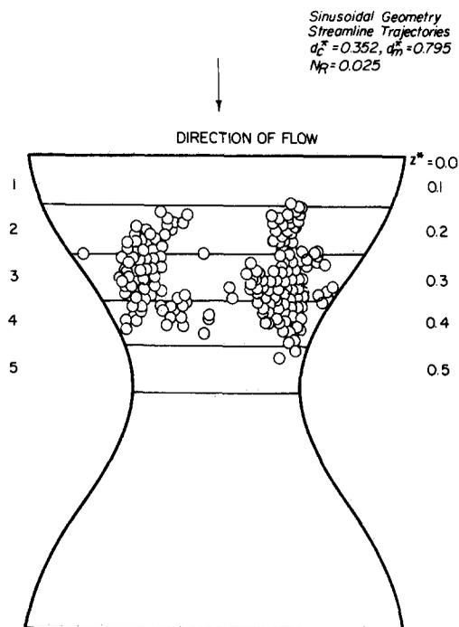
FIG. 12. Typical deposit pattern for streamline trajectories, side view.
