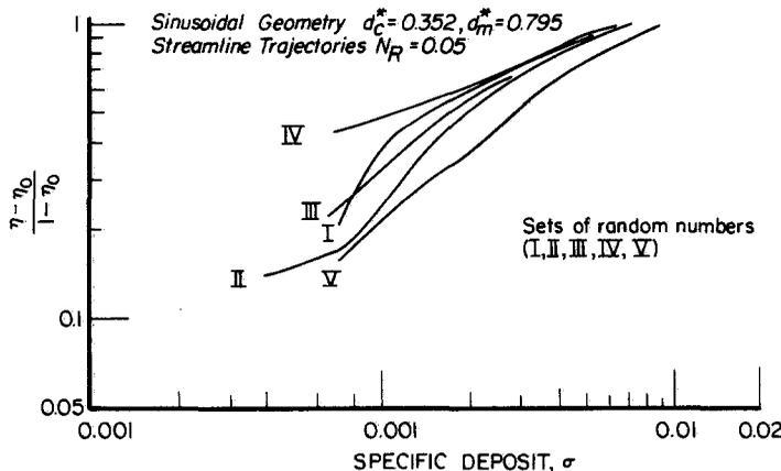
FIG. 3. Stochastic variability of simulation results,  $\eta$  vs  $\sigma$  data.
