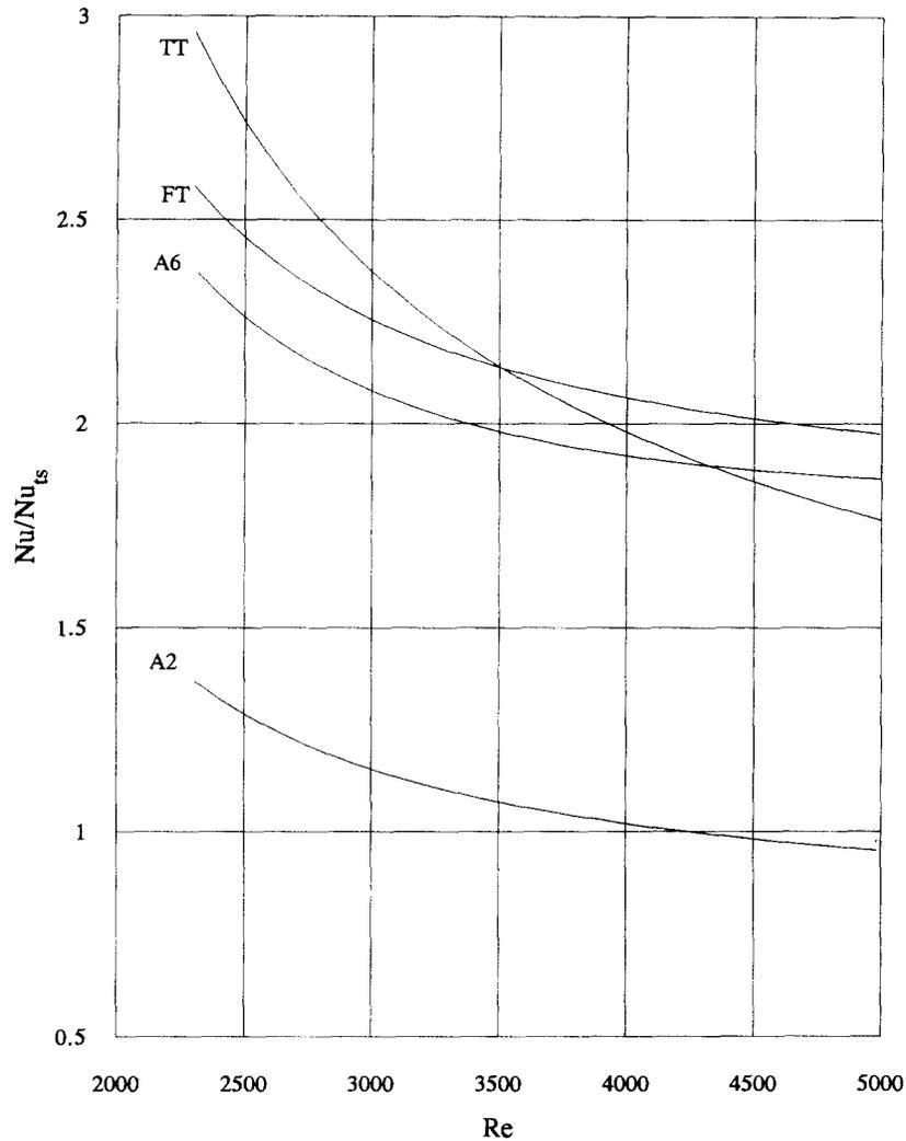
Fig. 9. Enhancement ratio for turbulent flow with equal pumping power.
