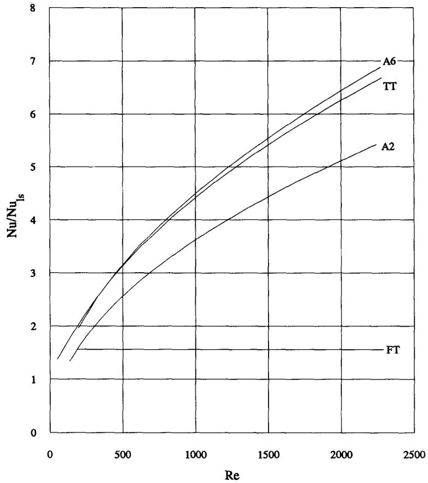
Fig. 8. Enhancement ratio for laminar (Darcy and Forchheimer) flow with equal pumping power.
