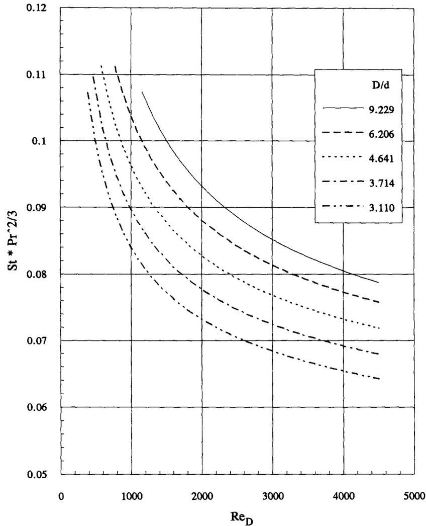
Fig. 6. Heat transfer characteristics in the turbulent regime per equation (30).
