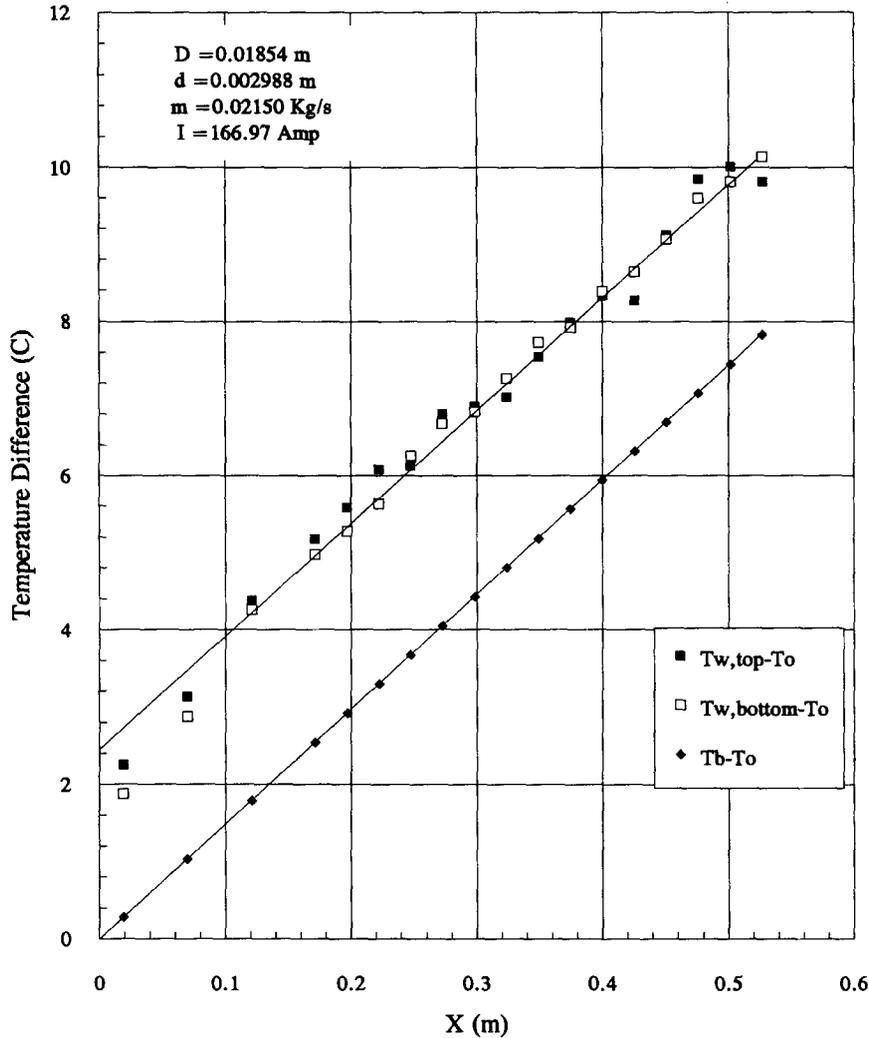
Fig. 2. Axial variation of wall and fluid temperatures for test A3.
