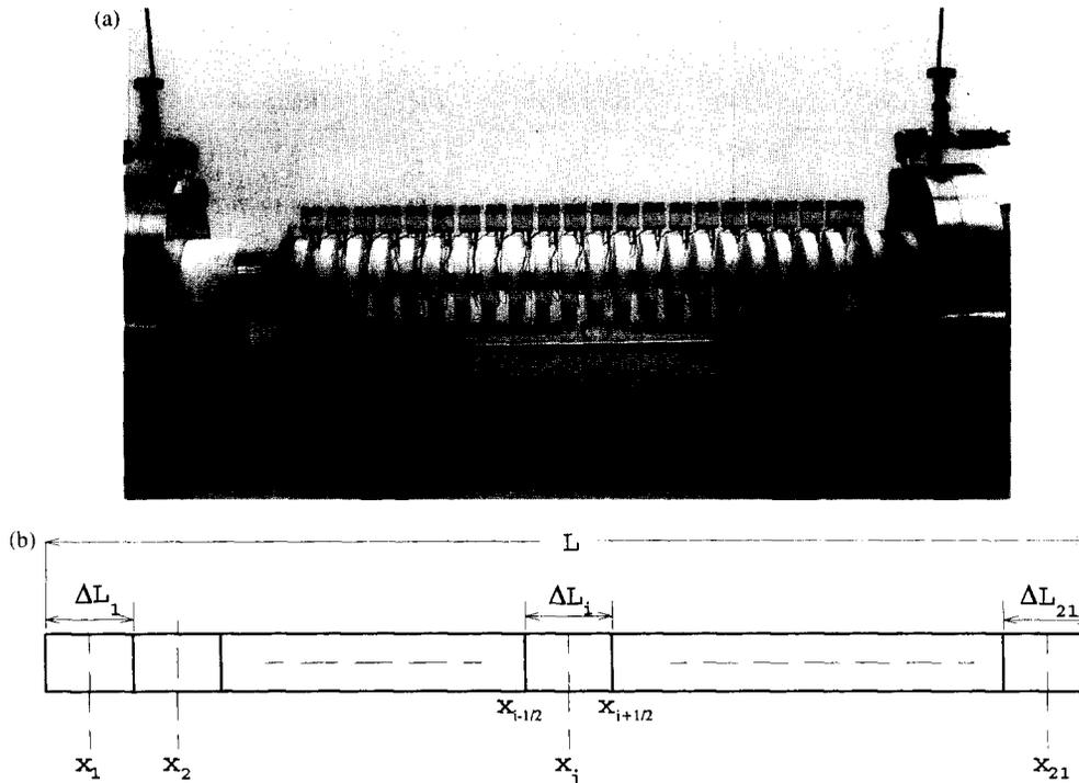
Fig. 1. Test section, (a) photograph of installed test section, (b) subdivision of test section for evaluating the local Nusselt number. Thermocouples were located at stations 1, 3, 5 and 7–21 at top and bottom of tubes.
