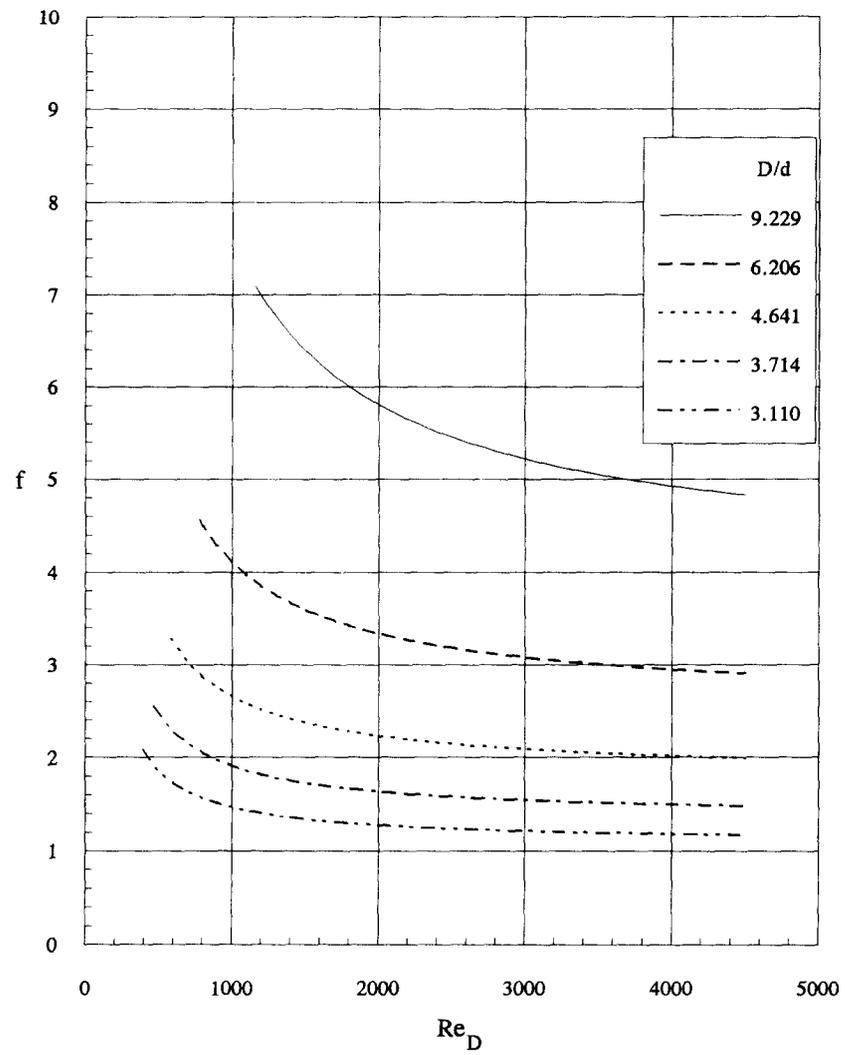
Fig. 7. Flow-friction characteristics in the turbulent regime per equation (31).
