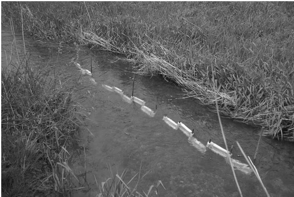
Several Teflon holders fixed in line at the stream bed
