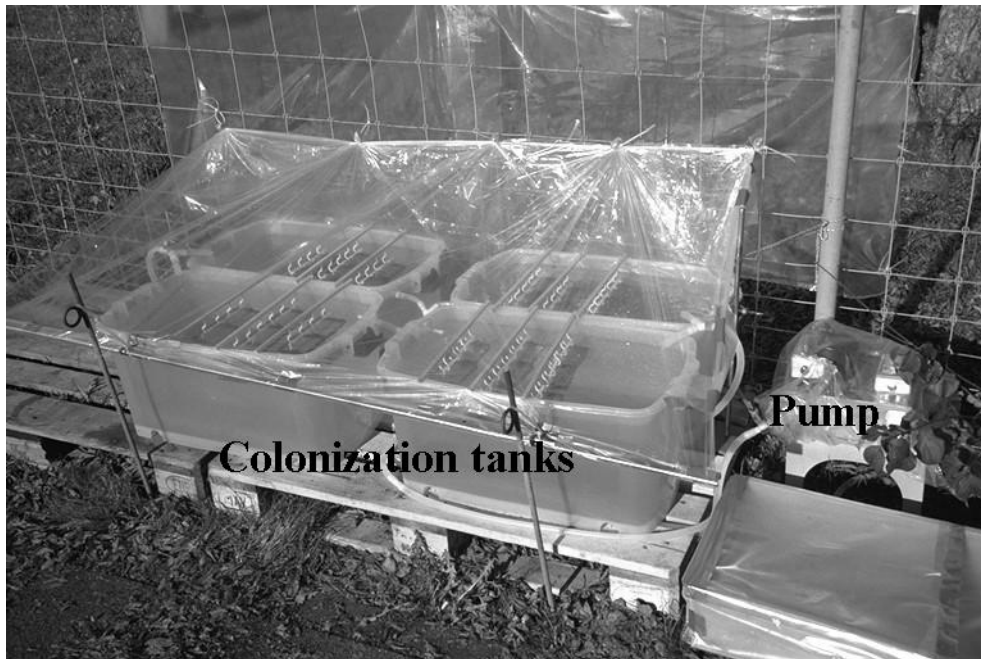
Tanks operated as a flow-through system and used for periphyton colonization
