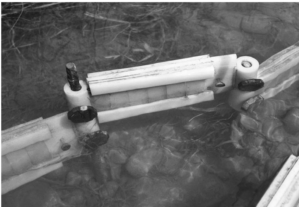
Periphytic biofilm growing on microscope slides fixed to Teflon holders
