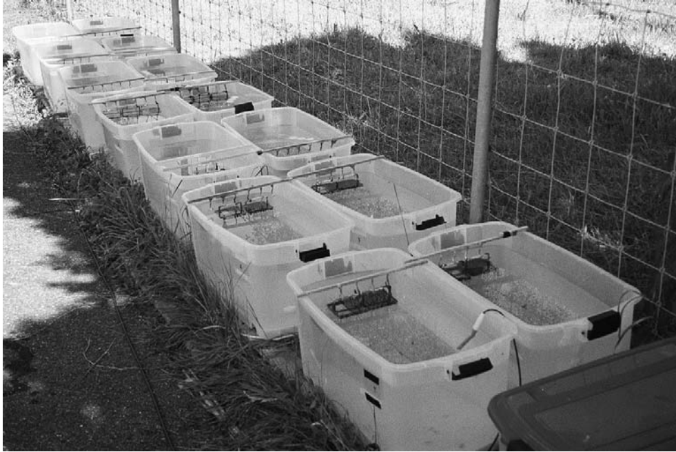
Experimental tanks with periphyton exposed to different metal speciation
