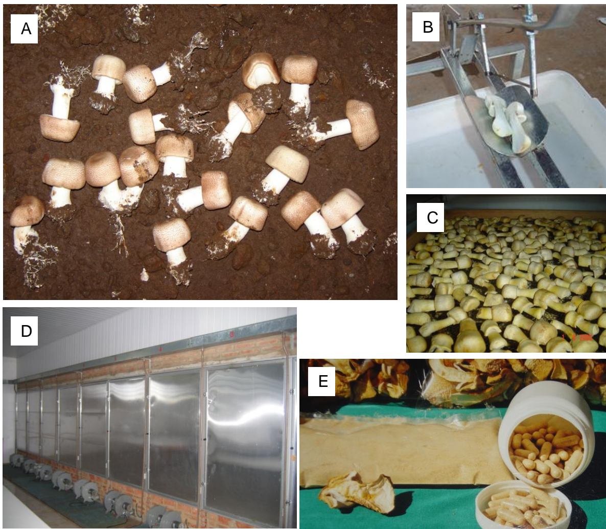
Figure 10. A: Freshly harvested mushrooms with residue of the casing layer and fragments of mycelium at the base of the stipe. B: Washed mushrooms cut in half showing brown color absent. C: Mushrooms in trays that are placed in a dehydrator. D: Mushroom dehydration room; each dehydrator (covered by aluminium door) has an electric resistance heating system and forced ventilation and has a capacity of 100 kg of mushrooms per day. E: Dehydrated mushrooms sliced in half (light color and without signs of oxidation, standard for export) and powder and capsules, ready to be marketed.
