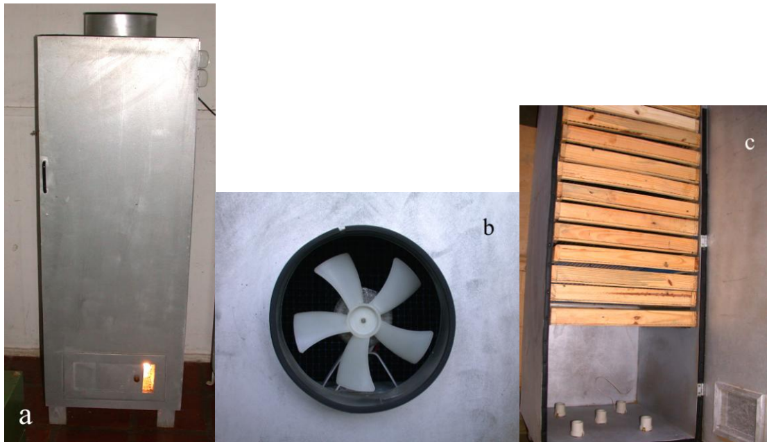
Figure 9. Electric dryer for shiitake. a: metallic cabinet, b: extraction fan, c: wooden trays for placement of mushrooms.
