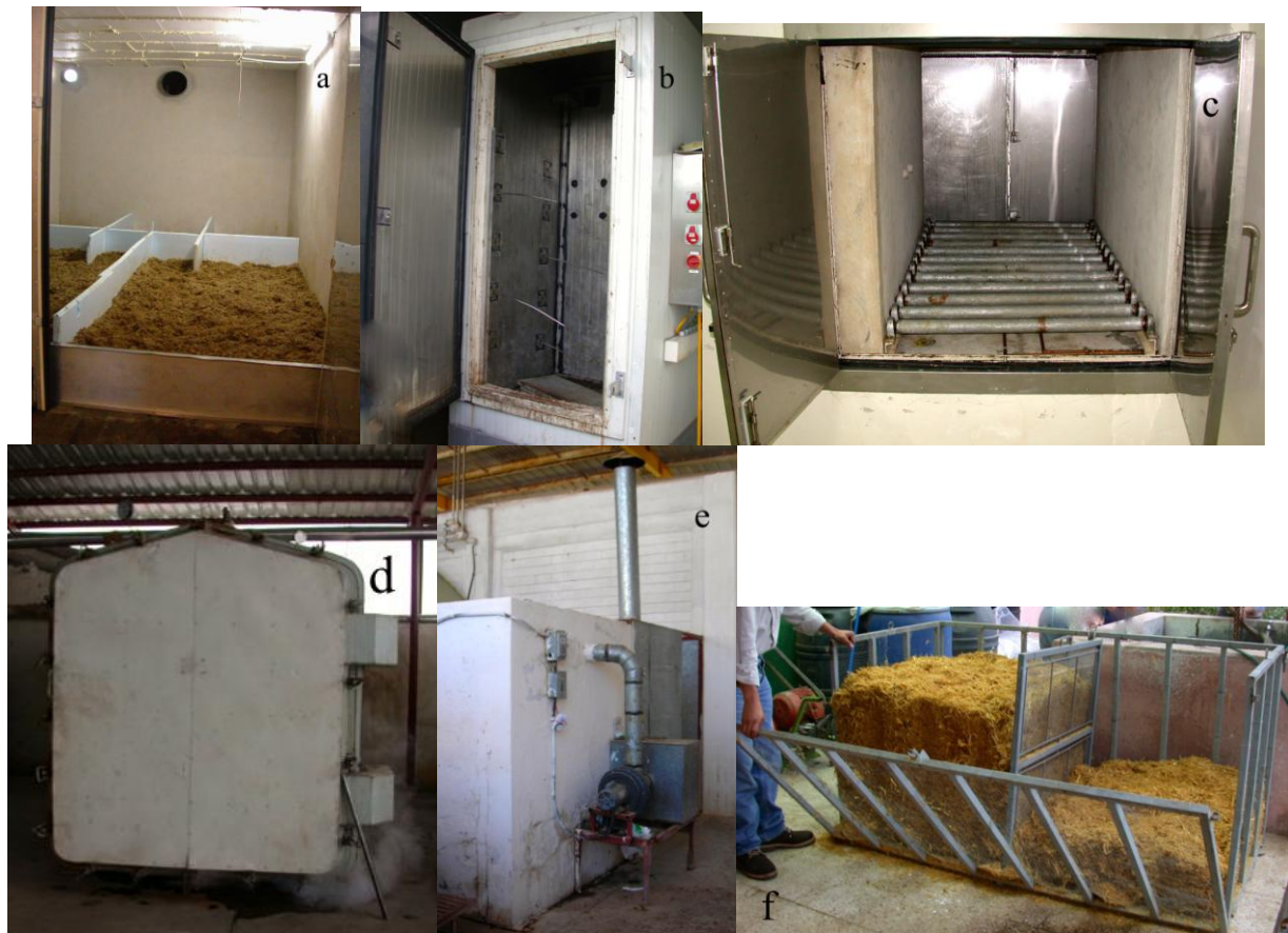
Figure 5. Different systems for straw pasteurization with steam. a: single-door pasteurization room for bulk substrate, b: pasteurization system type "box", c: pasteurization system of double door (outdoor-indoor), with rollers, for substrate in containers, d: single door pasteurization system for substrate in containers, e: detail of the motor for steam recirculation and air filter, f: metallic container for fermenting or pasteurizing straw.
